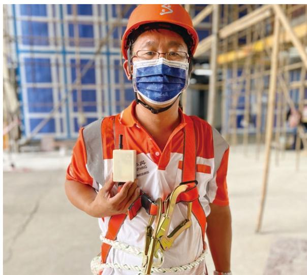
Automatic Detection System for Safety Harness
